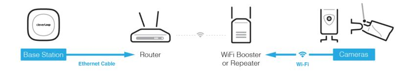
WiFi booster should be placed in between the router and the camera(s) for the maximum signal boosting outcome.
