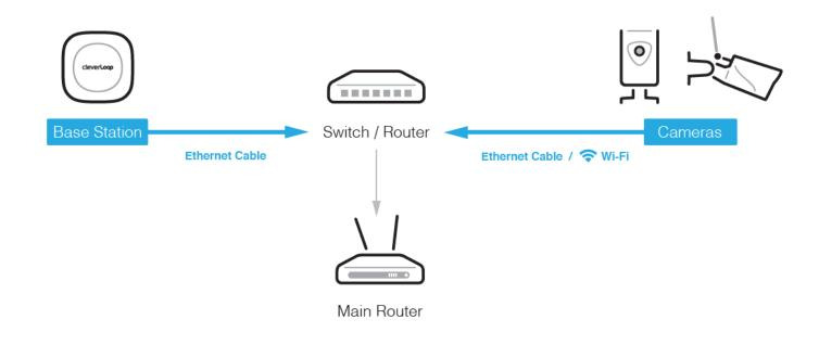
Base Station and the camera(s) should be connected to the **same** router / switch, otherwise the Base Station won't be able to find the camera(s).
